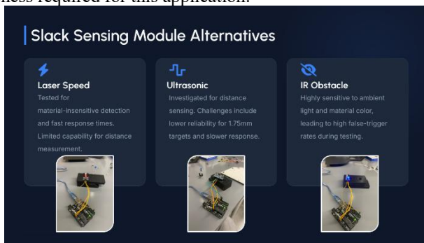
Fig. 9. Test setups and comparison of evaluated sensor modules
